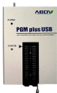
Figure 1-1 PGMplusUSB ( Single Writer )
