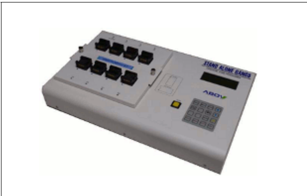
Figure 1-5 Standalone Gang8 (Gang Writer)
