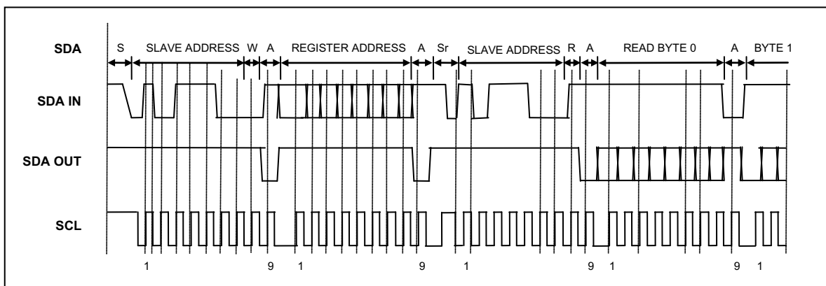
Figure 2-6 I2C Read Protocol
