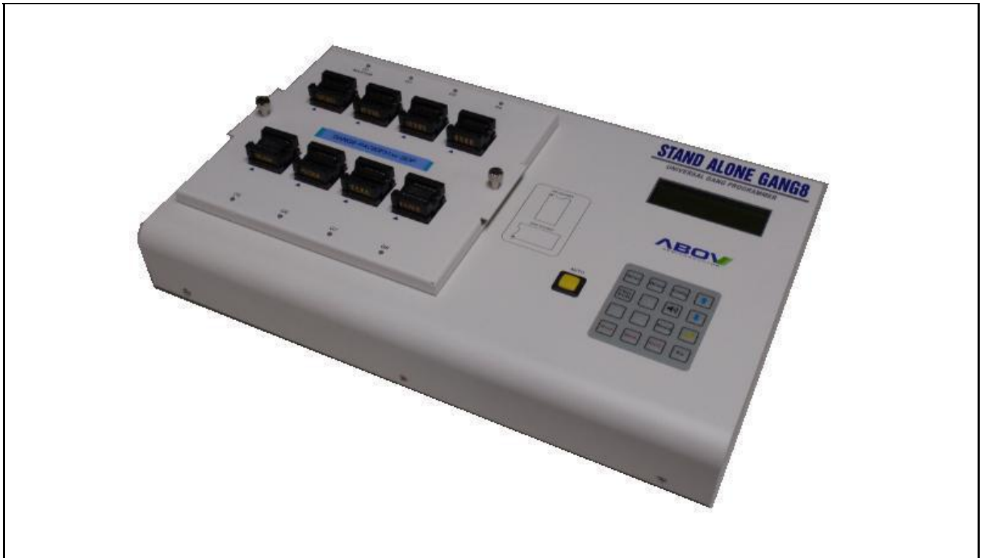
Figure 1.6 StandAlone Gang8 (for Mass Production)
