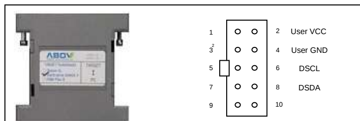
Figure 1.1 OCD Debugger and Pin Description
