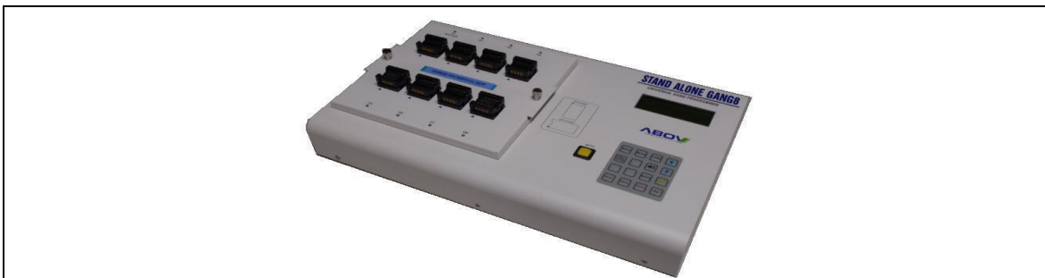
Figure 1.4 StandAlone Gang8 (for Mass Production)
