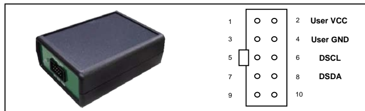
Figure 1-1 On Chip Debugger 2 and Pin description (ocd2 mode)
