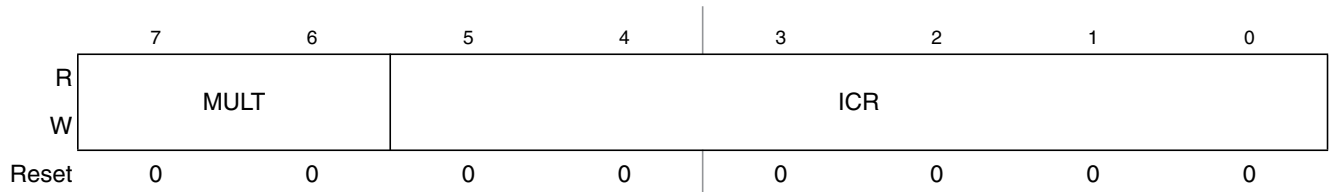
Figure 13-4. IIC Frequency Divider Register (IIC1F)
