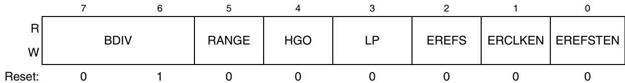
Figure 8-4. ICS Control Register 2 (ICSC2)
