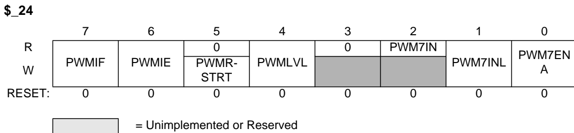
Figure 3-15 PWM Shutdown Register (PWMSDN)
