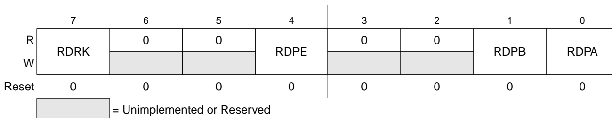
Figure 18-15. Reduced Drive Register (RDRIV)
