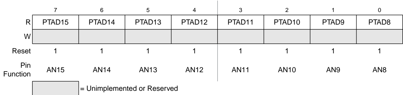
Figure 9-16. Port Data Register 0 (PORTAD0)
