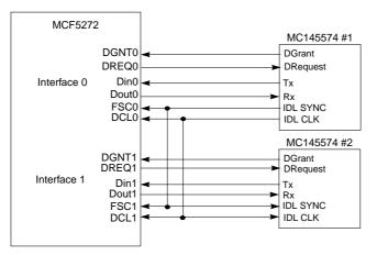
Figure 13-41. Two-Line Remote Access
