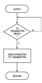
Figure 16-31. UART Mode Programming Flowchart (Sheet 5 of 5)
