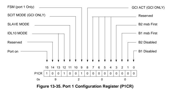
The programming of the P1CR register in the above example is achieved with the following ColdFire code sequence assuming the equates and init sections include the following:
