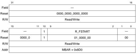
Figure 11-13. FIFO Receive Start Register (FRSR)
