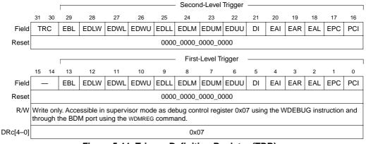
A write to TDR clears the CSR trigger status bits, CSR[BSTAT].
