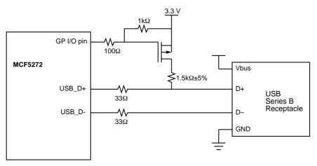
Figure 12-24. Recommended USB Line Interface
