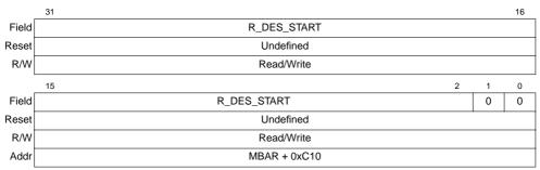
Figure 11-23. Pointer to Receive Descriptor Ring (ERDSR)
