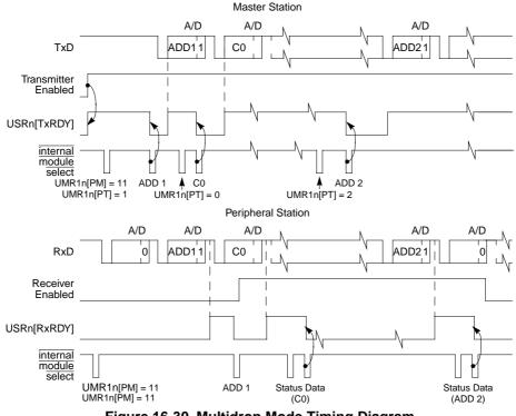
Figure 16-30. Multidrop Mode Timing Diagram
