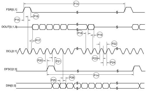
Figure 23-18 shows IDL slave timings listed in Table 23-18.
