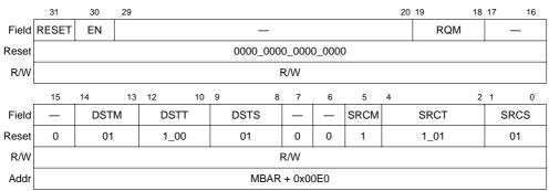
Figure 10-1. DMA Mode Register (DMR)
