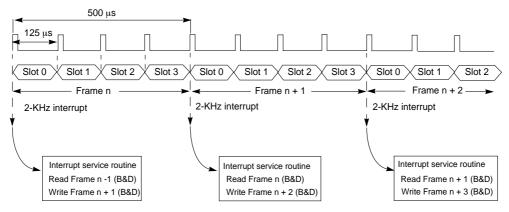
Figure 13-10. Periodic Frame Interrupt
