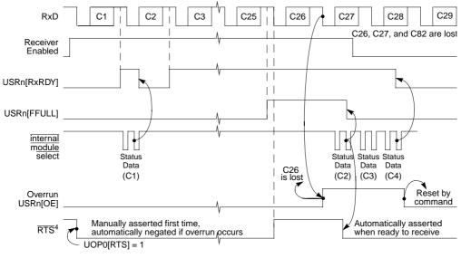
Figure 16-26. Receiver Timing
