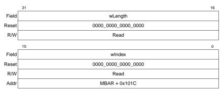
Figure 12-10. USB Device Request Data 2 Register (DRR2)
