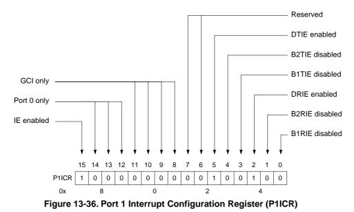
The programming of the P1ICR in the above example is achieved with the following ColdFire code sequence assuming the equates and init sections as in the previous P1CR example:
