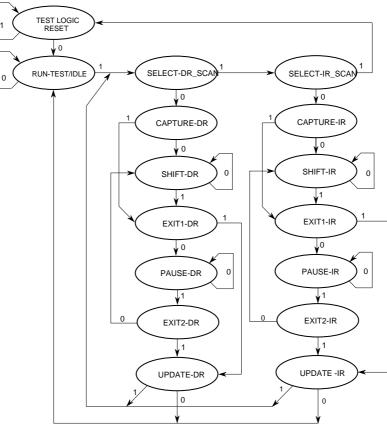
Figure 21-2. TAP Controller State Machine
