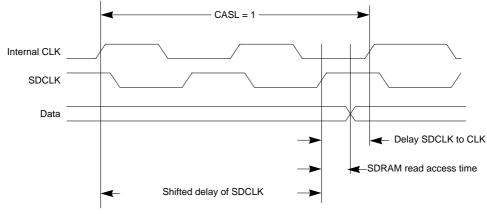
$T_{SDCLK to CLK}$  -  $T_{acc}$  > 0 => effective CAS latency reduced by 1
