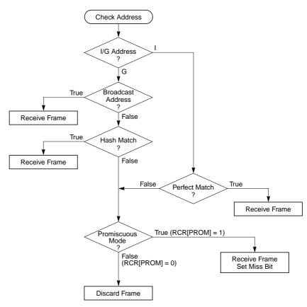
Figure 11-4. Ethernet Address Recognition Flowchart
