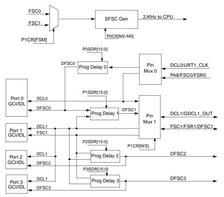
Figure 13-11. PLIC Internal Timing Signal Routing
