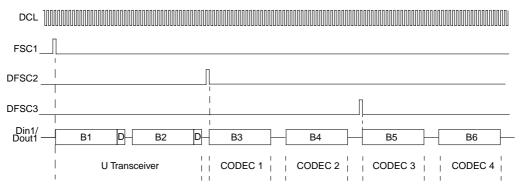
Figure 13-40. Standard IDL2 10-bit mode.
