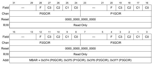
Figure 13-28. GCI C/I Channel Receive Registers (P0GCIR–P3GCIR)
