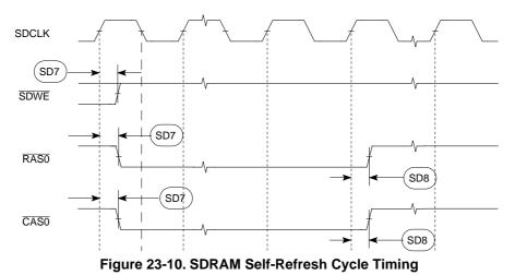
Figure 23-10 shows SDRAM self-refresh timings listed in Table 23-10.
