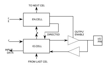
NOTE: More than one IO.Cell could be serially connected and controlled by a single En.Cell.
