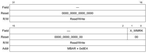
Figure 11-14. Transmit FIFO Watermark (TFWR)
