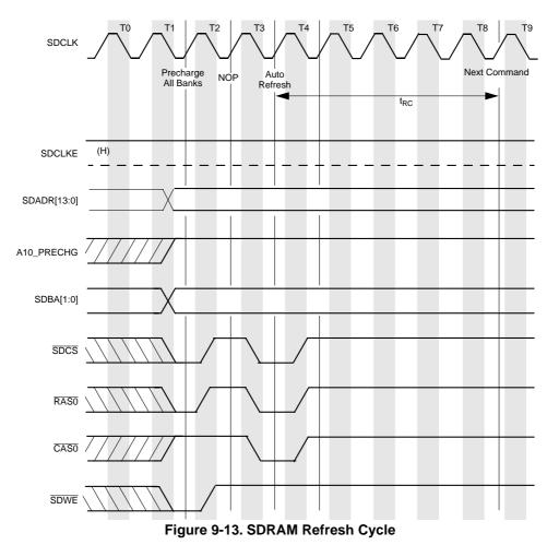
Figure 9-14 shows the timing for entering SDRAM self-refresh mode. During a PRECHARGE ALL command (T1), the SDRAM writes all of its on-chip RAM page buffers back into the SDRAM array. The SDTR[RP] value determines the number of dead cycles after a precharge. Note that auto refresh occurs in T3. SDTR[RC] determines the number of clock cycles the SDRAM remains in refresh state, during which time it cannot accept
