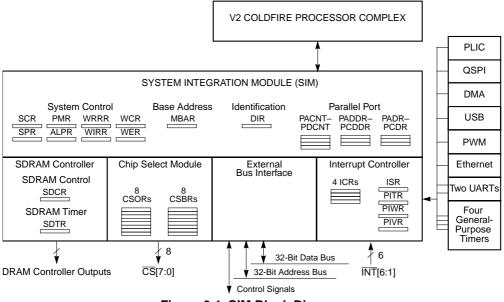
Figure 6-1. SIM Block Diagram
