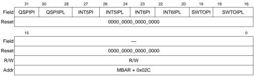
Figure 7-5. Interrupt Control Register 4(ICR4)
