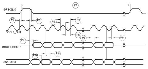
Figure 23-17 shows IDL master timings listed in Table 23-17.
