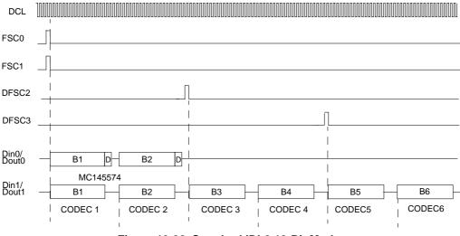
Figure 13-38. Standard IDL2 10-Bit Mode
