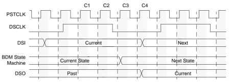
Figure 5-12. BDM Serial Interface Timing
