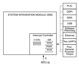
Figure 7-1. Interrupt Controller Block Diagram
