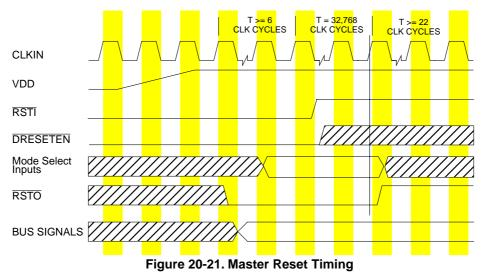
When the assertion of  $\overline{\text{RSTI}}$  is recognized internally, the MCF5272 asserts the reset out pin ( $\overline{\text{RSTO}}$ ). The  $\overline{\text{RSTO}}$  pin is asserted as long as  $\overline{\text{RSTI}}$  is asserted and remains asserted for 32,768 CLKIN cycles after  $\overline{\text{RSTI}}$  is negated.
