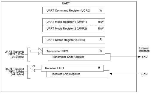
Figure 16-24. Transmitter and Receiver Functional Diagram
