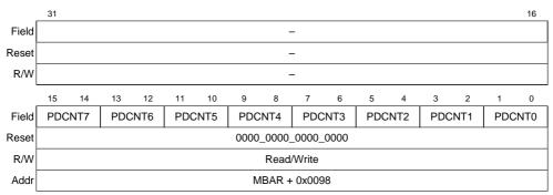
Figure 17-3. Port D Control Register (PDCNT)
