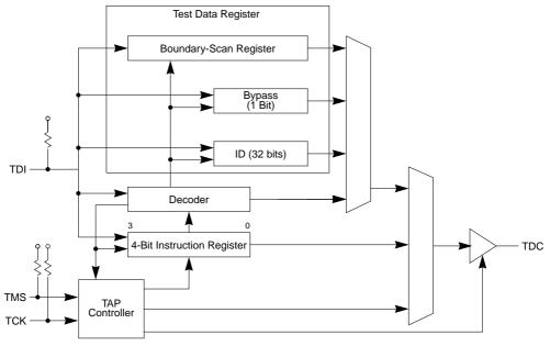
Figure 21-1. Test Access Port Block Diagram
