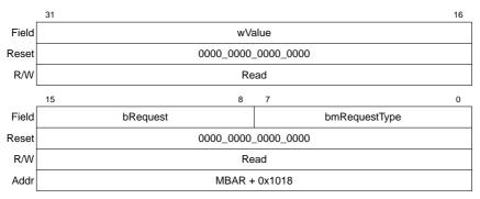
Figure 12-9. USB Device Request Data 1 Register (DRR1)
