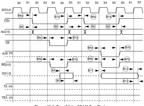
Figure 23-3. Read/Write SRAM Bus Timing
