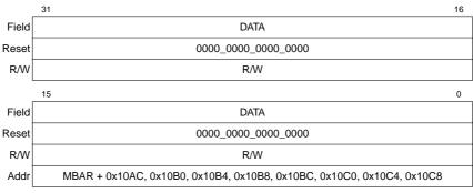
Figure 12-21. USB Endpoint 0-7 Data Registers (EPnDR)
