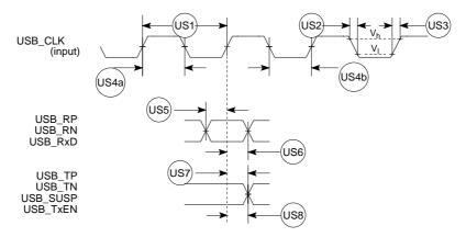
Figure 23-22. USB Interface Timing
