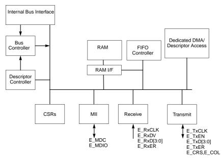
Figure 11-2. Fast Ethernet Module Block Diagram
