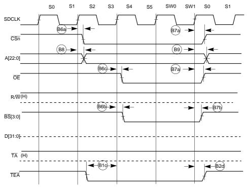
Figure 23-5. SRAM Bus Cycle Terminated by TEA
