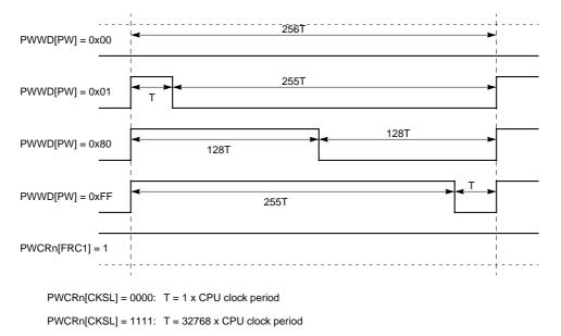
Figure 18-4. PWM Waveform Examples (PWCR*n*[EN] = 1)
