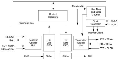
Figure 11-1. Ethernet Block Diagram
