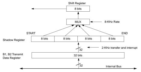
Figure 13-5. GCI/IDL B Data Transmit Register Multiplexing
