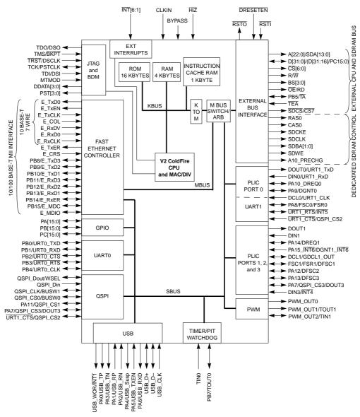
NOTE: GPIO pins shown above are multiplexed with most other signals.
