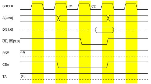
Figure 20-3. Longword Read; EBI = 00; 32-Bit Port; Internal Termination
