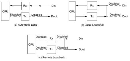
Figure 13-9. GCI/IDL Loopback Mode
