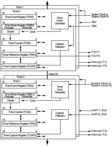
Figure 15-1. Timer Block Diagram
