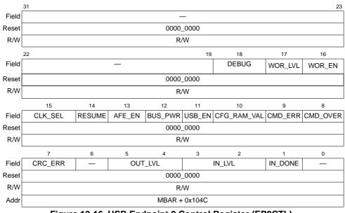
Figure 12-16. USB Endpoint 0 Control Register (EP0CTL)
