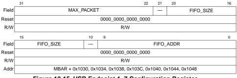
Figure 12-15. USB Endpoint 1–7 Configuration Register
