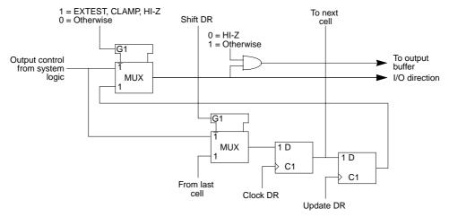
Figure 21-5. Output Control Cell (En.Cell) (BC-4)
