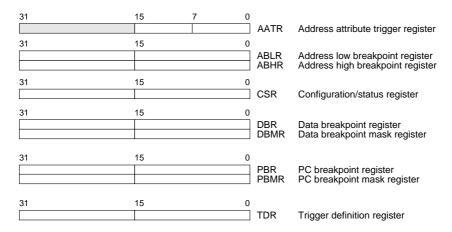
Note: Each debug register is accessed as a 32-bit register; shaded fields above are not used (don't care). All debug control registers are writable from the external development system or the CPU via the WDEBUG instruction.
