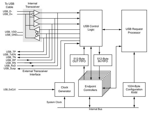
Figure 12-2. USB Module Block Diagram
