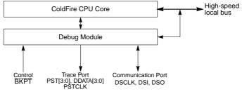
Figure 5-1. Processor/Debug Module Interface
