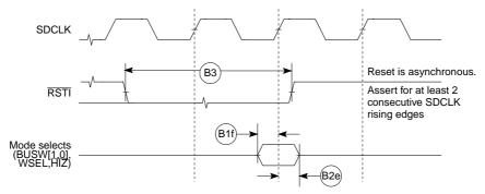
Figure 23-6. Reset and Mode Select/HIZ Configuration Timing
