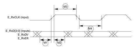
Figure 23-11. MII Receive Signal Timing Diagram
