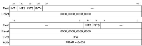
Figure 7-7. Programmable Interrupt Transition Register (PITR)
