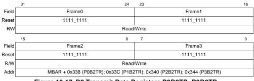
Figure 13-17. B2 Transmit Data Registers P0B2TR-P3B2TR
