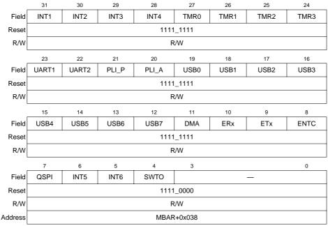
Figure 7-8. Programmable Interrupt Wakeup Register (PIWR)
