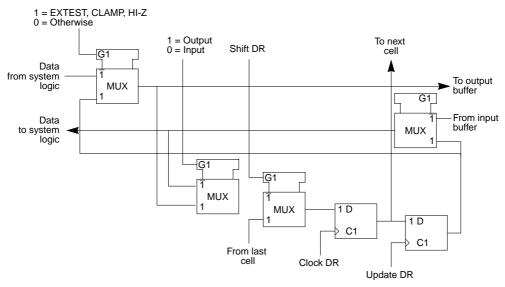
Figure 21-6. Bidirectional Cell (IO.Cell) (BC-6)
