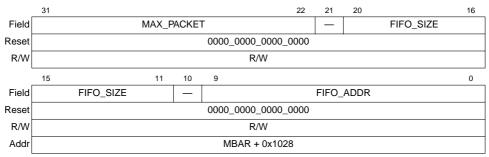
Figure 12-13. USB Endpoint 0 IN Configuration Register (IEP0CFG)
