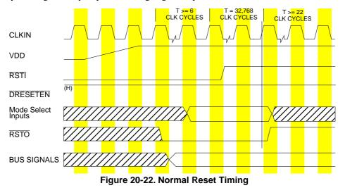
The levels of the mode select inputs, QSPI\_Dout/WSEL, QSPI\_CLK/BUSW1, QSPI\_CS0/BUSW0, and  $\overline{\text{HiZ}}$  are sampled when  $\overline{\text{RSTO}}$  negates and select the port size of  $\overline{\text{CS0}}$  and the physical data bus width after a master reset occurs.  $\overline{\text{RSTO}}$  is asserted as long
