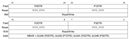
Figure 13-18. D Transmit Data Registers P0DTR–P3DTR
