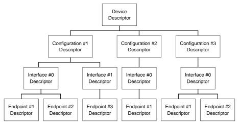
Figure 12-23. Example USB Configuration Descriptor Structure
