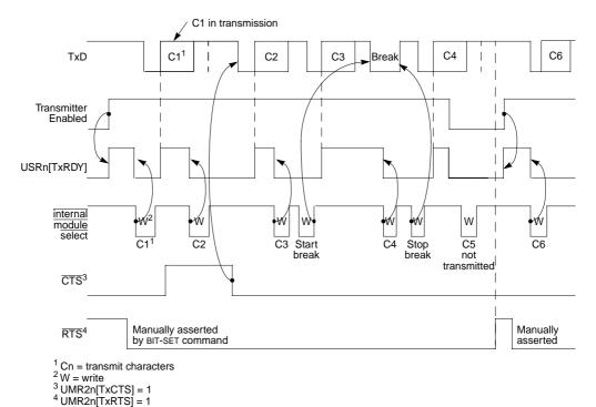
Figure 16-25 shows the functional timing information for the transmitter.
