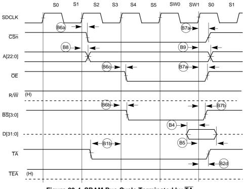
Figure 23-4. SRAM Bus Cycle Terminated by TA
