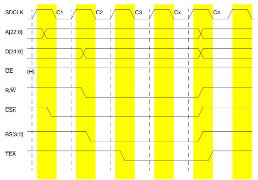
Figure 20-20. Longword Write Access To 32-Bit Port Terminated with TEA Timing
