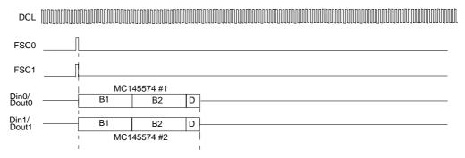
Figure 13-42. Standard IDL2 8-Bit mode
