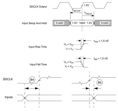
Figure 23-2. General Input Timing Requirements
