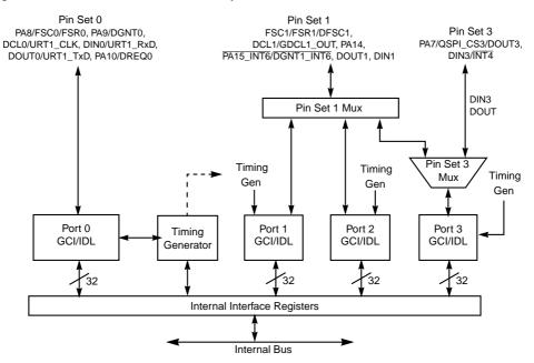
Figure 13-1 illustrates the basic PLIC system.
