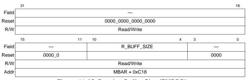
Figure 11-25. Receive Buffer Size (EMRBR)
