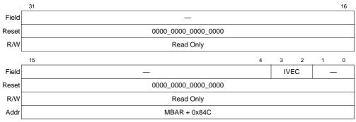
Figure 11-7. Interrupt Vector Status Register (IVSR)
