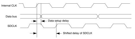
Figure 9-6. Timing Refinement with Inverted SDCLK
