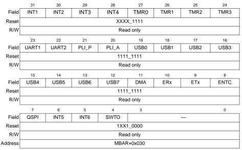
Figure 7-6. Interrupt Source Register (ISR)
