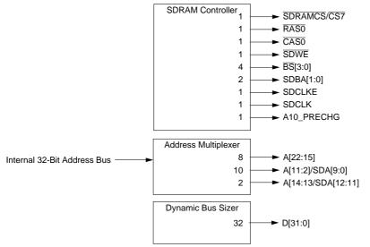
Figure 9-1 shows the SDRAM controller signal configuration.
