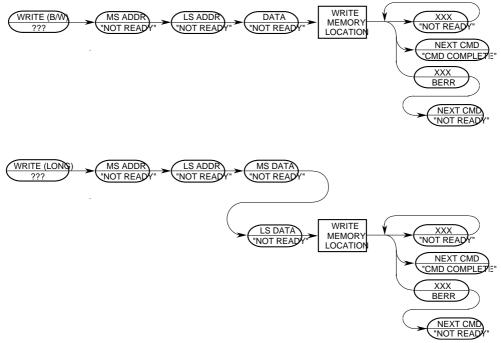
Figure 5-24. WRITE Command Sequence
