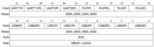
Figure 7-3. Interrupt Control Register 2 (ICR2)
