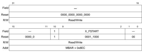
The TFSR register is reset to the first available RAM address.
