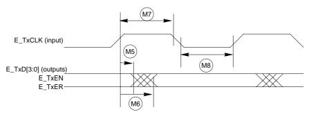
Figure 23-12. MII Transmit Signal Timing Diagram
