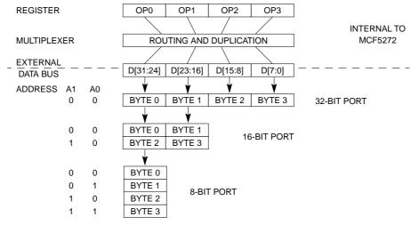
Figure 20-2. MCF5272 Interface to Various Port Sizes
