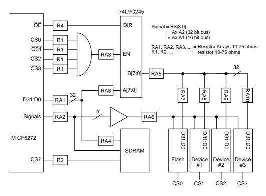
Figure B-1. Buffering and Termination
