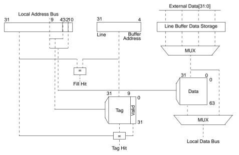
Figure 4-3. Instruction Cache Block Diagram
