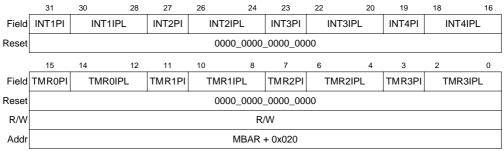
Figure 7-2. Interrupt Control Register 1 (ICR1)
