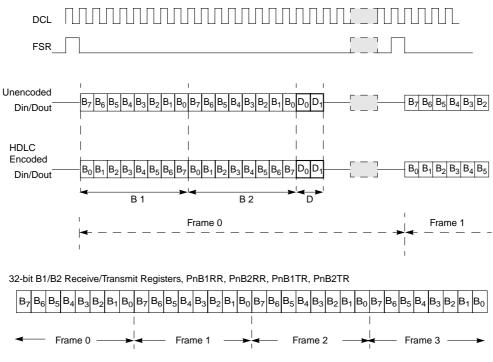
Figure 13-6. B-Channel Unencoded and HDLC Encoded Data
