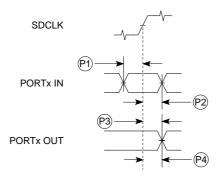
Figure 23-21. General-Purpose I/O Port Timing
