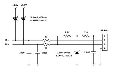
Figure 12-25. USB Protection Circuit
