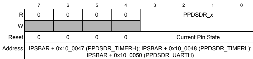
Figure 12-21. Port Pin Data/Set Data Registers (PPDSDR_x)
