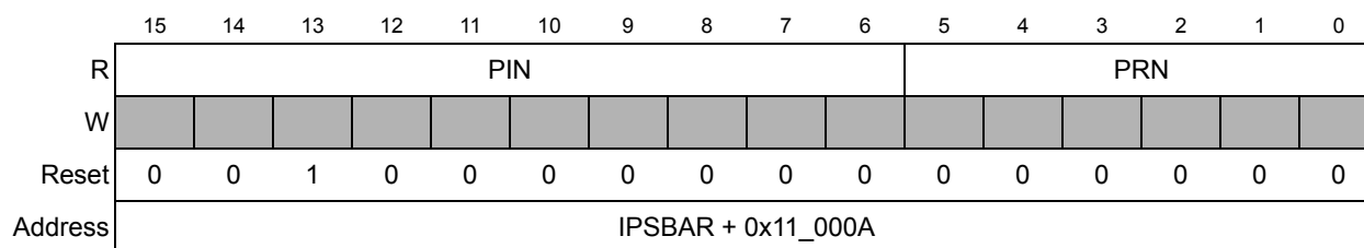
Figure 9-4. Chip Identification Register (CIR)
