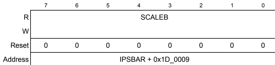
Figure 22-9. PWM Scale B Register (PWMSCLB)
