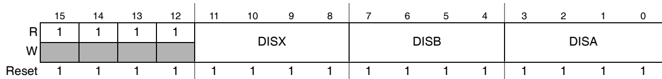
Figure 34-12. Fault Disable Mapping Register (PWM_SMnDISMAP)
