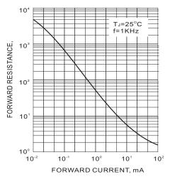
Fig.2-DYNAMIC FORWARD RESISTANCE VERSUS FORWARD CURRENT
