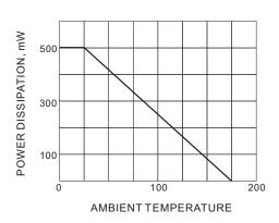
Fig.4 DERATING CURVE
