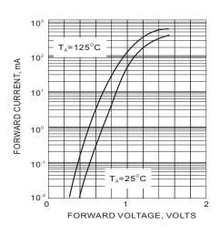
Fig.3 FORWARD CHARACTERISTICS
