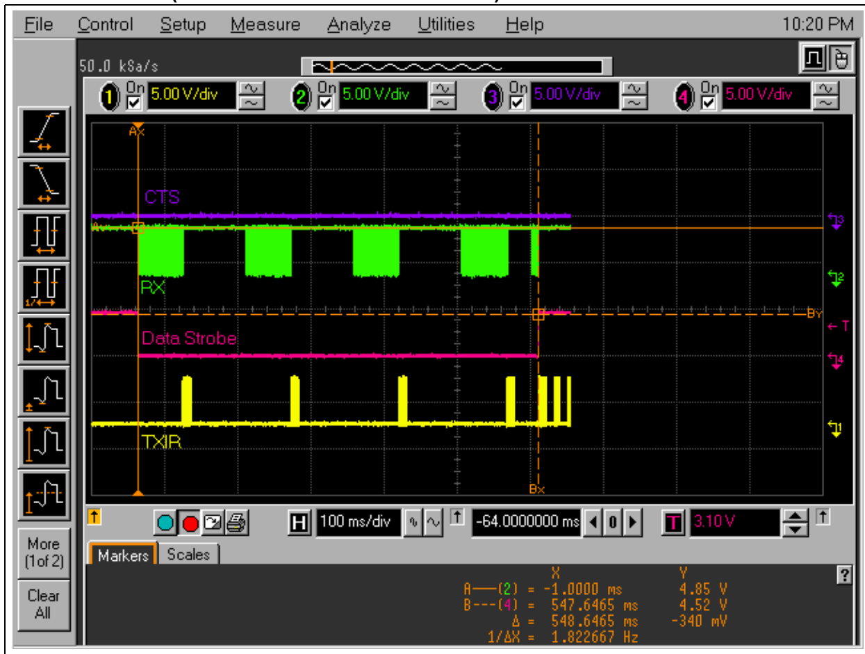
FIGURE 2-13: HOST CONTROLLER RECEPTION (P → S) OF A 250 BYTE PACKET (FROM PIC IRDA STANDARD STACK)
