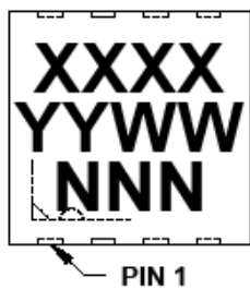
8-Lead DFN (3x3 mm)
