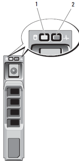
1 hard-drive activity indicator (green) 2 hard-drive status indicator (green and amber)
