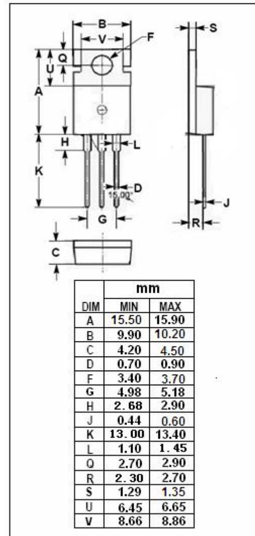
**isc N-Channel MOSFET Transistor****MDP1921****ELECTRICAL CHARACTERISTICS**T<sub>C</sub>=25°C unless otherwise specified
