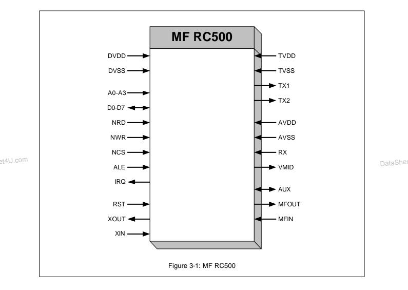
The device operates with 3 individual power supplies for best performance in terms of EMC behaviour and signal de-coupling. This gives outstanding RF performance and also maximum flexibility to adapt to different operating voltages of digital and analog part.
