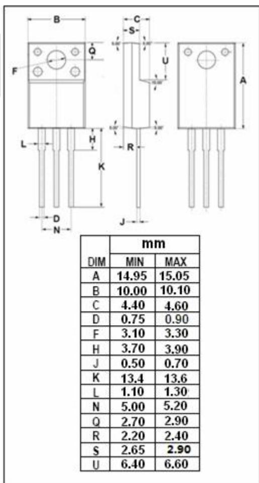
**isc N-Channel MOSFET Transistor****MFT60N12T22FS****• ELECTRICAL CHARACTERISTICS (T<sub>c</sub>=25°C)**
