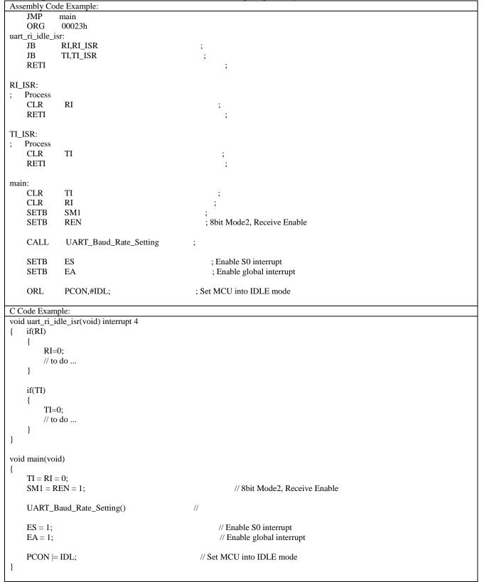
(1). Required Function: IDLE mode with RI wake-up capability
