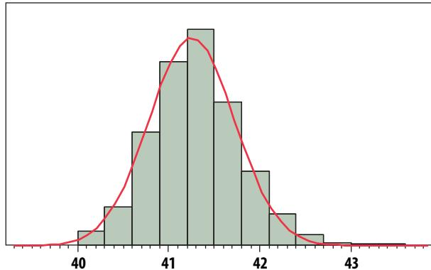
Figure 5. OIP3 @ 900MHz, V<sub>dd</sub> = 5V, LSL = 38.2, Nominal = 41.8dBm
