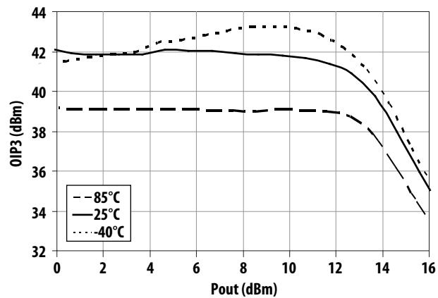
Figure 14. OIP3 vs Output Power and Temperature
