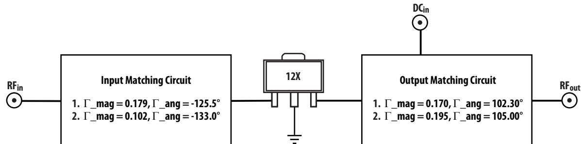
Figure 27. Input and output tuned Gamma location for 1900MHz<sup>(1)</sup>, 2500MHz<sup>(2)</sup>
