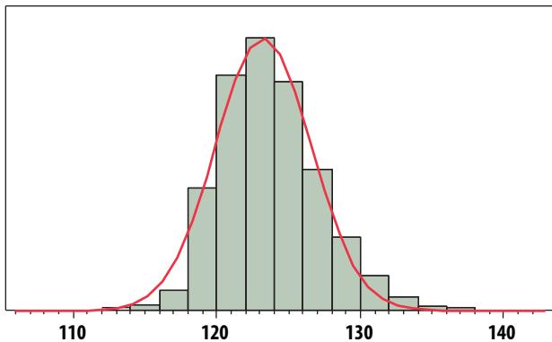
Figure 2. I<sub>DD</sub> @ 1900MHz, V<sub>dd</sub> = 5V, LSL = 101mA, Nominal = 124mA, USL = 143mA
