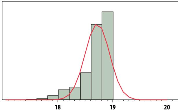
Figure 4. Gain @ 900MHz, V<sub>dd</sub> = 5V, LSL = 17dB, Nominal = 18.7dB, USL = 20dB
