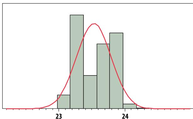
Figure 6. P1dB @ 900MHz, V<sub>dd</sub> = 5V, LSL = 21.8dBm, Nominal = 23.6dBm
