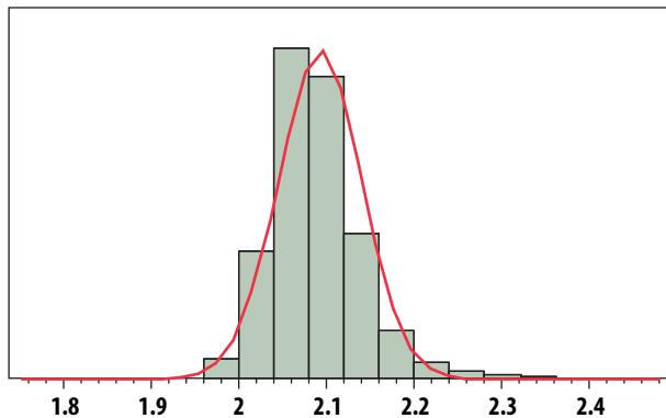
Figure 3. NF @ 900MHz, V<sub>dd</sub> = 5V, Nominal = 2dB, USL = 2.45dB
