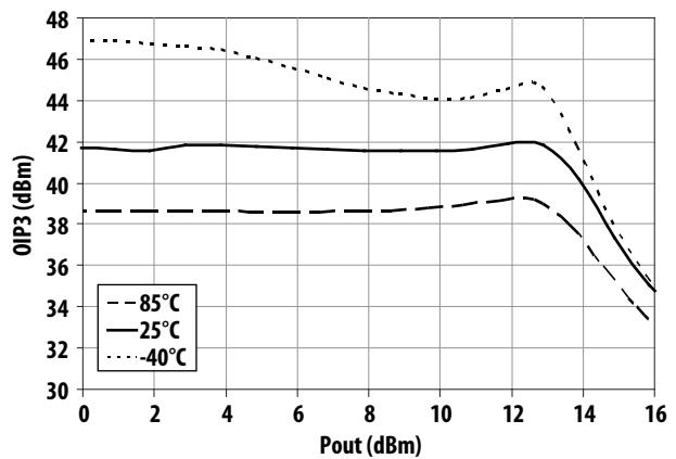
Figure 23. OIP3 vs Output Power and Temperature
