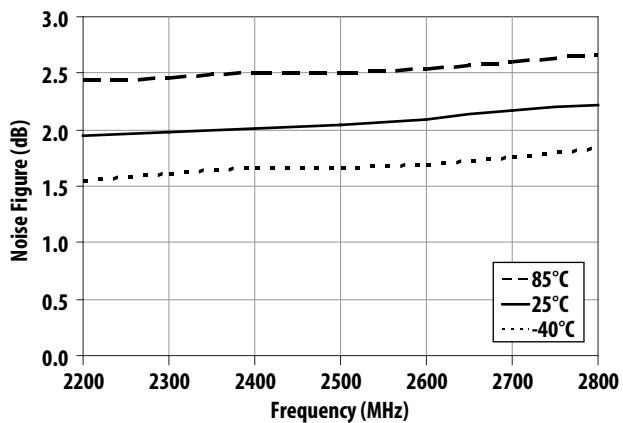
Figure 22. Noise Figure vs Frequency and Temperature
