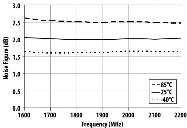
Figure 13. Noise Figure vs Frequency and Temperature
