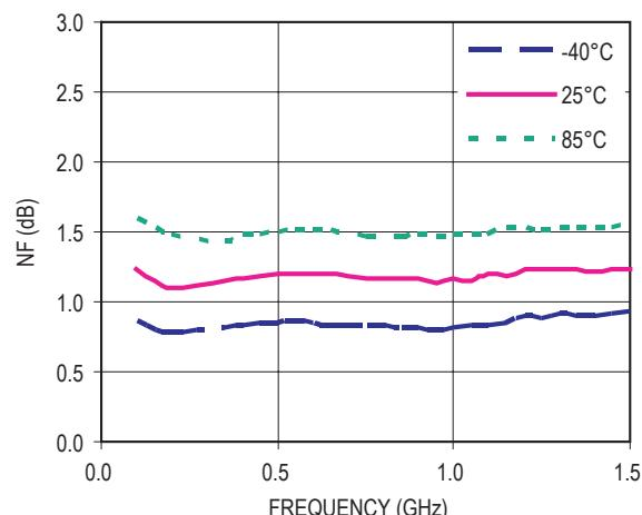
Figure 30. NF vs Frequency ( $V_d = 5V$ ,  $I_{ds} = 5mA$ )
