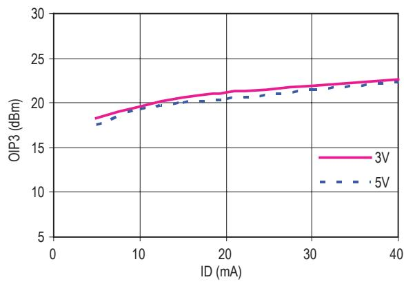
Figure 50. OIP3 vs Id ( 100 MHz )
