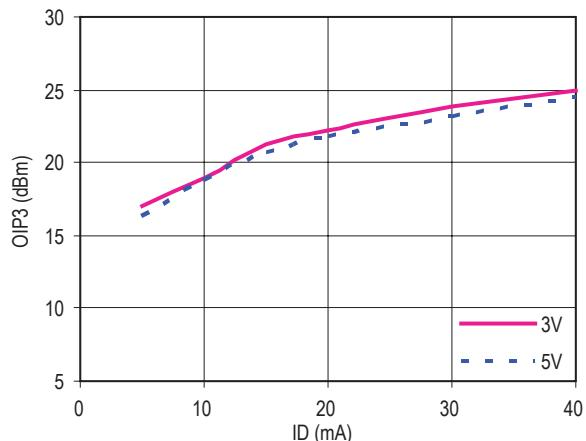
Figure 46. OIP3 vs Id ( 500 MHz )
