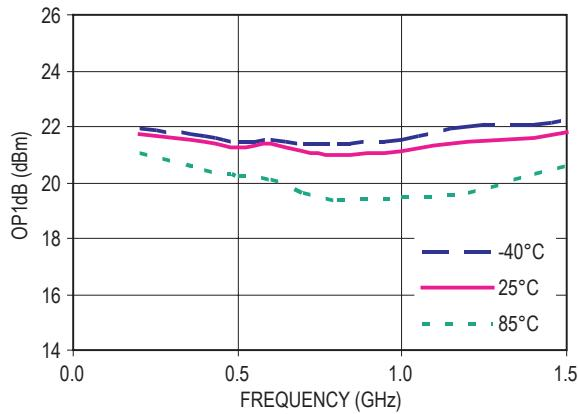
Figure 33. OP1dB vs Frequency ( $V_d = 5V$ ,  $I_{ds} = 10mA$ )
