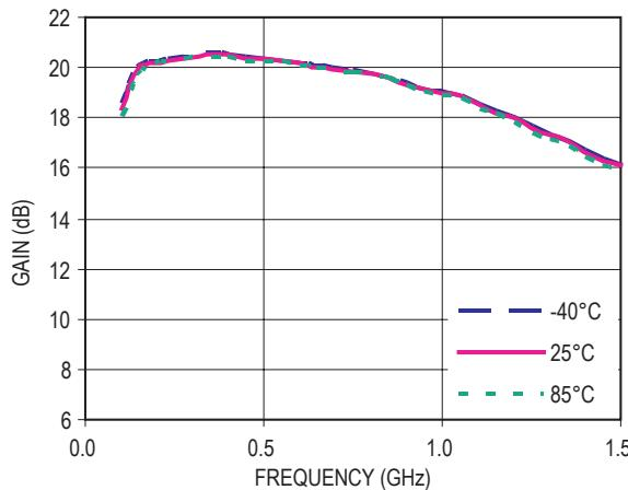
Figure 41. Gain vs Frequency ( $V_d = 5V$ ,  $I_{ds} = 15mA$ )
