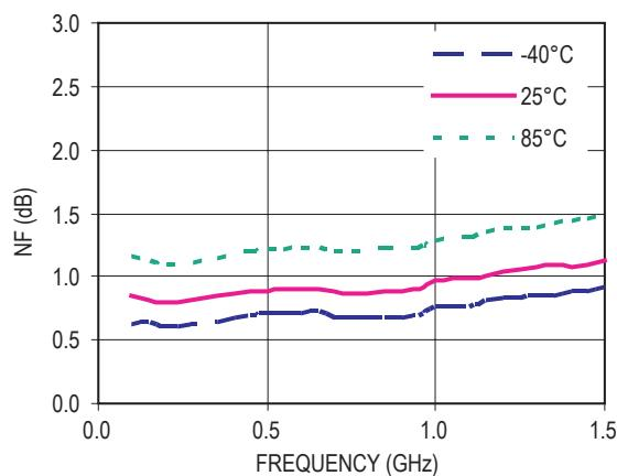
**Figure 24. NF vs Frequency ( $V_d = 3V$ ,  $I_{ds} = 15mA$ )**
