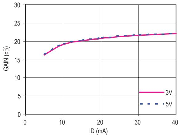
Figure 47. Gain vs Id( 500 MHz )
