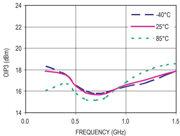
Figure 7. OIP3 vs Frequency ( $V_d = 3V$ ,  $I_{ds} = 5mA$ )
