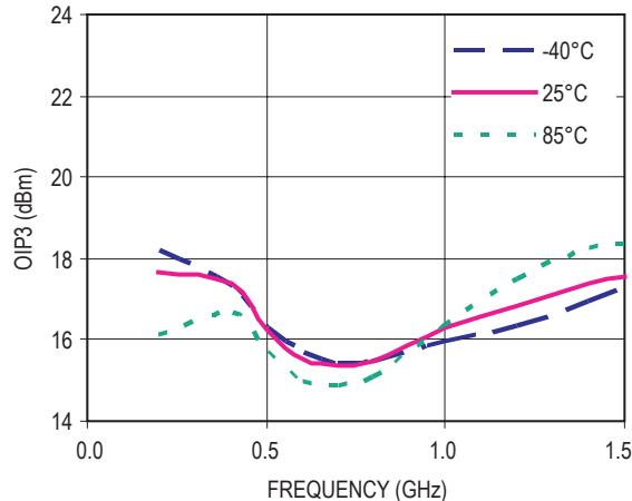
Figure 28. OIP3 vs Frequency ( $V_d = 5V$ ,  $I_{ds} = 5mA$ )
