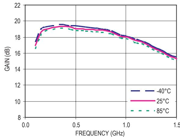
Figure 14. Gain vs Frequency ( $V_d = 3V$ ,  $I_{ds} = 10mA$ )
