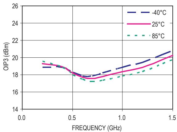
Figure 34. OIP3 vs Frequency ( $V_d = 5V$ ,  $I_{ds} = 10mA$ )
