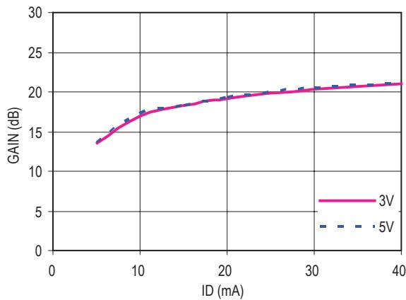
**Figure 51. Gain vs Id( 100 MHz )**
