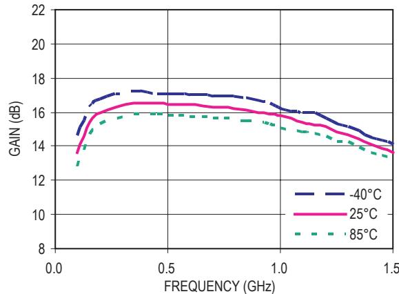
Figure 8. Gain vs Frequency ( $V_d = 3V$ ,  $I_{ds} = 5mA$ )
