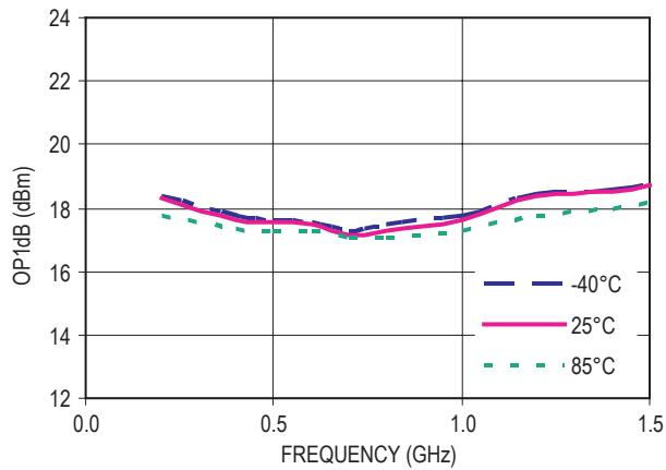
Figure 20. OP1dB vs Frequency ( $V_d = 3V$ ,  $I_{ds} = 10mA$ )
