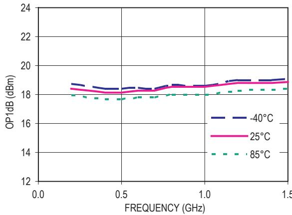
Figure 6. OP1dB vs Frequency ( $V_d = 3V$ ,  $I_{ds} = 5mA$ )
