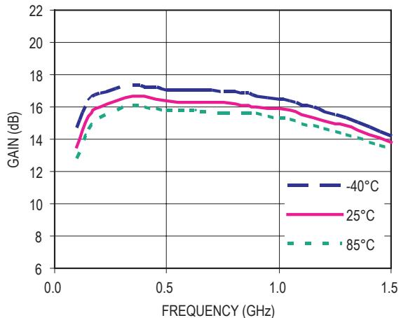
Figure 29. Gain vs Frequency ( $V_d = 5V$ ,  $I_{ds} = 5mA$ )
