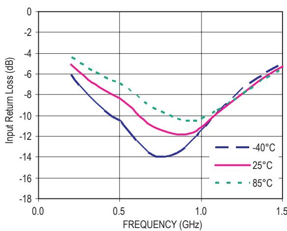
Figure 37. Input Return Loss vs Frequency ( $V_d = 5V$ ,  $I_{ds} = 10mA$ )
