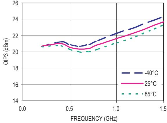
Figure 40. OIP3 vs Frequency ( $V_d = 5V$ ,  $I_{ds} = 15mA$ )
