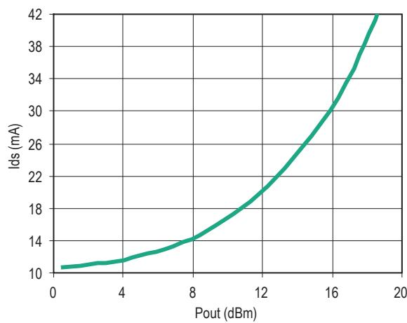
**Figure 53. Ids vs Pout (Vd = 3V)**
