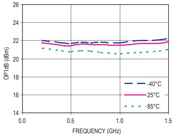
Figure 27. OP1dB vs Frequency ( $V_d = 5V$ ,  $I_{ds} = 5mA$ )
