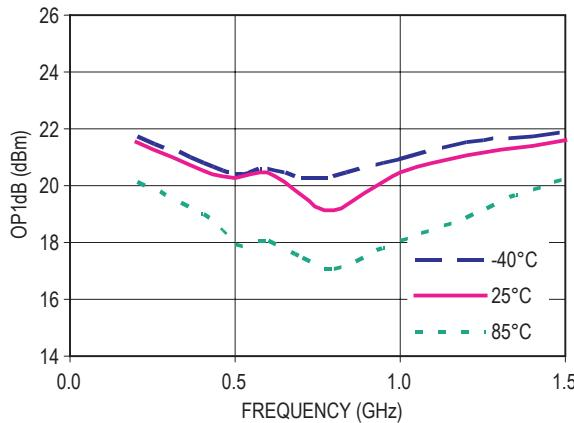
Figure 39. OP1dB vs Frequency ( $V_d = 5V$ ,  $I_{ds} = 15mA$ )
