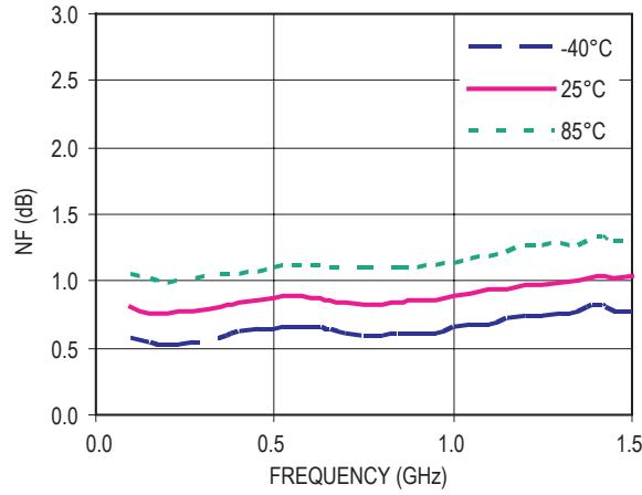
Figure 42. NF vs Frequency ( $V_d = 5V$ ,  $I_{ds} = 15mA$ )
