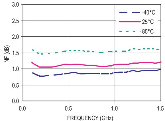
Figure 9. NF vs Frequency ( $V_d = 3V$ ,  $I_{ds} = 5mA$ )
