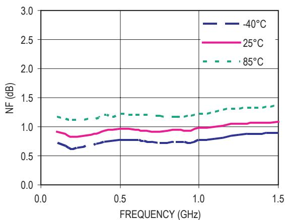
Figure 36. NF vs Frequency ( $V_d = 5V$ ,  $I_{ds} = 10mA$ )
