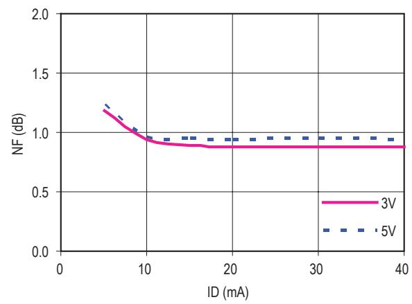
Figure 48. NF vs Id ( 500 MHz )
