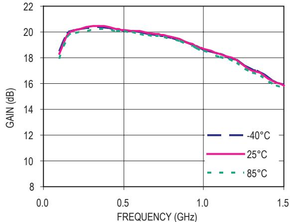
**Figure 23. Gain vs Frequency ( $V_d = 3V$ ,  $I_{ds} = 15mA$ )**
