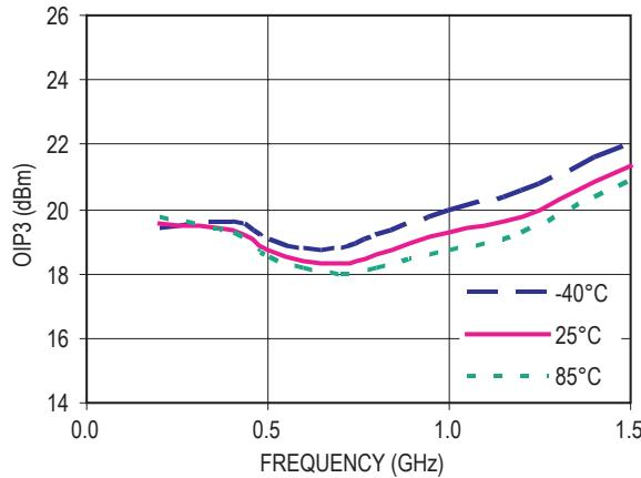
Figure 12. OIP3 vs Frequency ( $V_d = 3V$ ,  $I_{ds} = 10mA$ )
