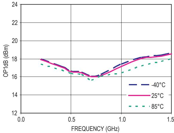
**Figure 21. OP1dB vs Frequency ( $V_d = 3V$ ,  $I_{ds} = 15mA$ )**
