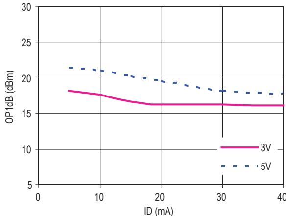
Figure 45. OP1dB vs Id ( 500 MHz )
