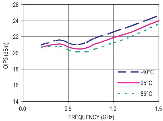
**Figure 22. OIP3 vs Frequency ( $V_d = 3V$ ,  $I_{ds} = 15mA$ )**
