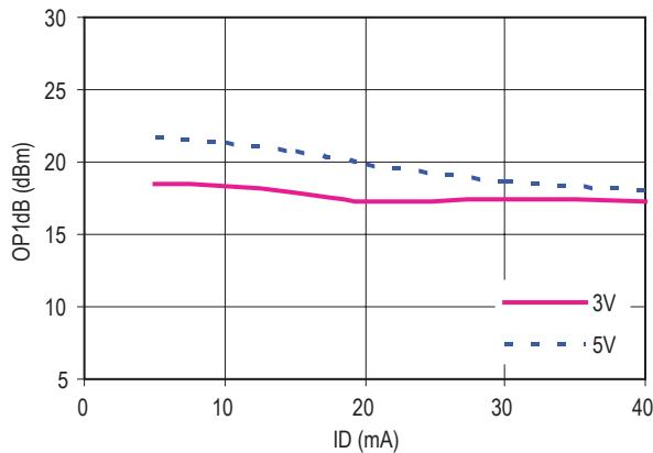
Figure 49. OP1dB vs Id ( 100 MHz )
