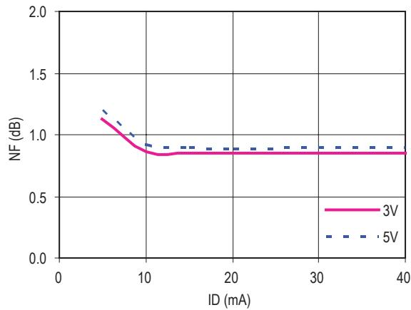
**Figure 52. NF vs Id ( 100 MHz )**
