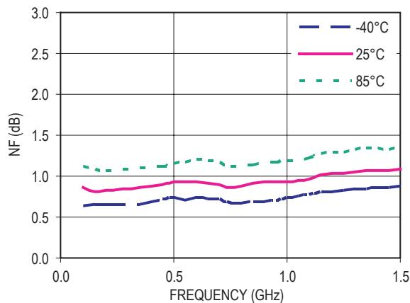
Figure 16. NF vs Frequency ( $V_d = 3V$ ,  $I_{ds} = 10mA$ )
