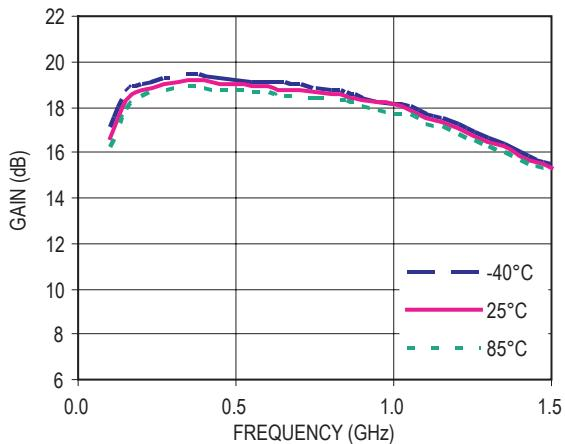
Figure 35. Gain vs Frequency ( $V_d = 5V$ ,  $I_{ds} = 10mA$ )
