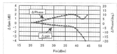
Test Condition : Vds=12V, Idq=4A, Ta=25deg.C
