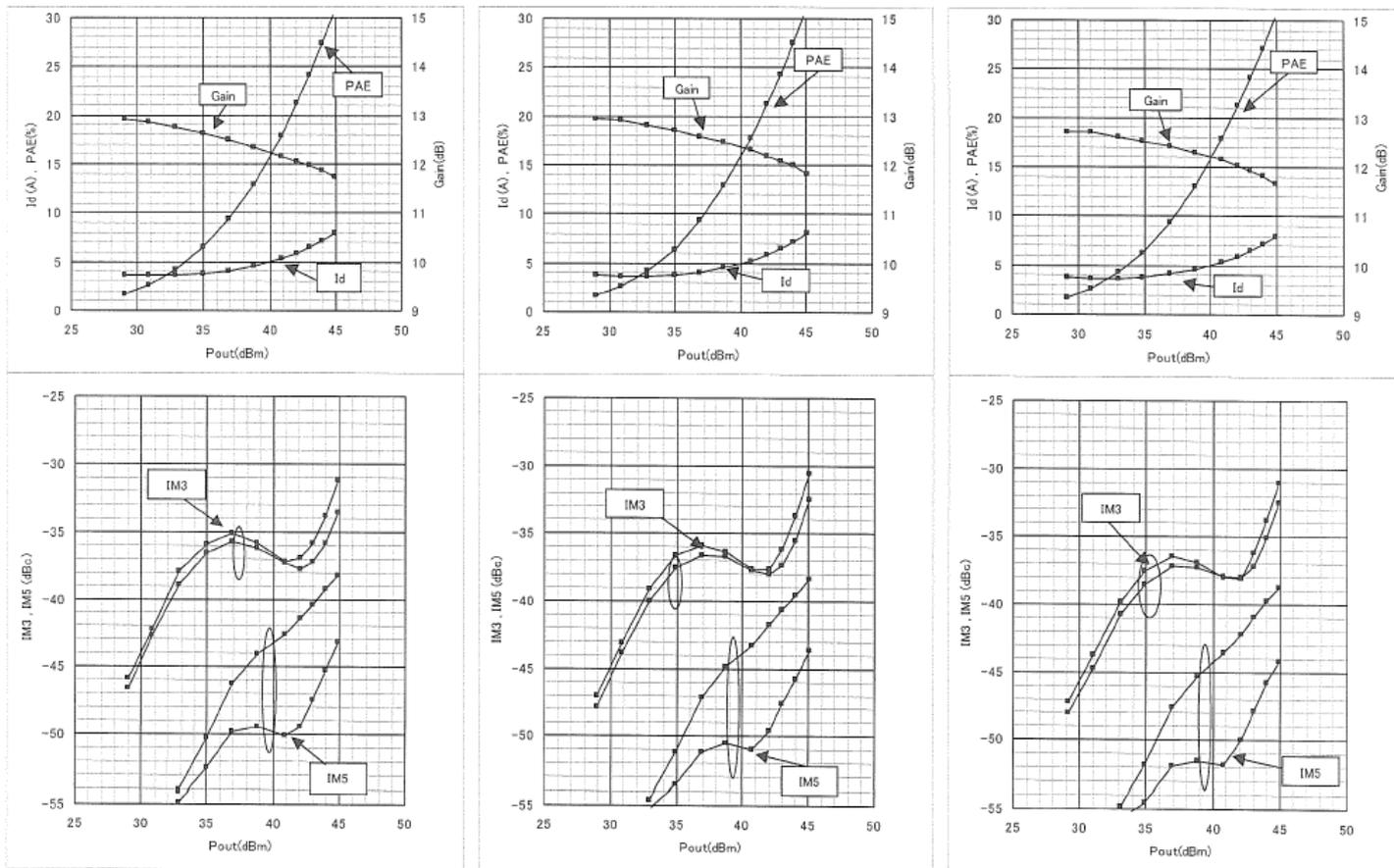
Test Condition : Vds=12V, Idq=4A, Ta=25deg.C
