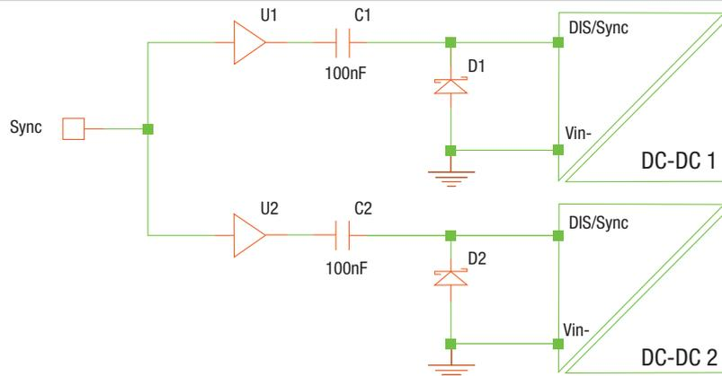
1. A suggested synchronisation circuit is shown. C1 and C2 are 100nF capacitors. D1 and D2 are schottky diodes. The capacitive coupling and close connected diode ensures that a transition from high to low is seen at the input pin even in a noisy environment or when there is a slight ground shift between devices.
