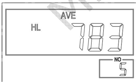
**Note:** Use a calibrated hardness tester, test the standard test block downward vertically for 5 times, the arithmetical average value compare with the value of standard test block. If this value exceeds the standard value, could use the function of user calibration to adjust.
