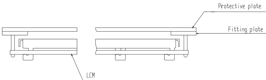
4.1.2 When assembling the LCM into other equipment, the spacer to the bit between the LCM and the fitting plate should have enough height to avoid causing stress to the module surface, refer to the individual specifications for measurements. The measurement tolerance should be  $\pm 0.1$ mm.
