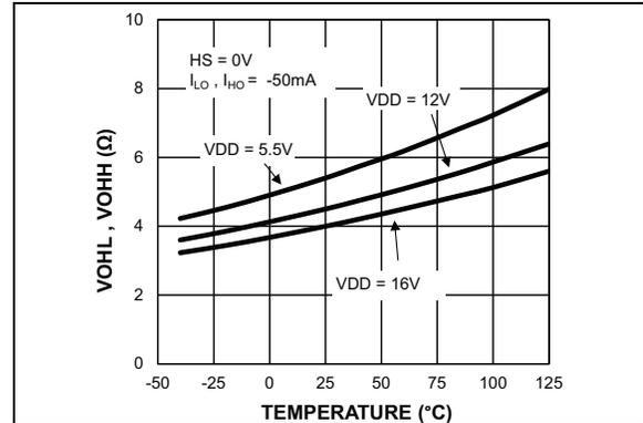
**FIGURE 3-10:** High Level Output Resistance vs. Temperature.
