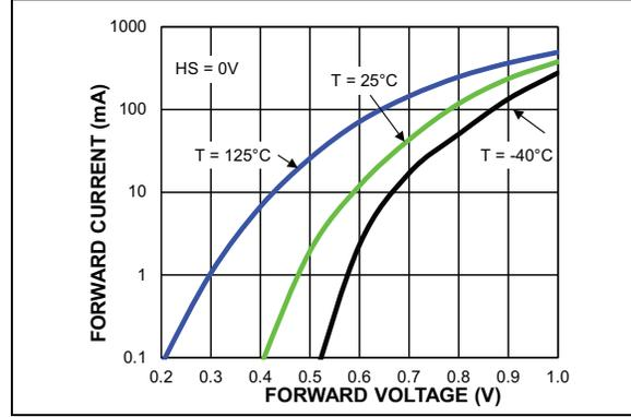
**FIGURE 3-18:** Bootstrap Diode I-V Characteristics.
