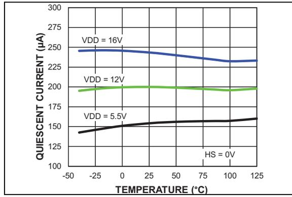
**FIGURE 3-6:**  $V_{DD}$  Quiescent Current vs. Temperature.
