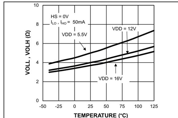
**FIGURE 3-11:** Low Level Output Resistance vs. Temperature.
