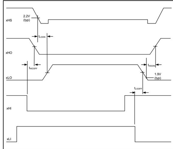
**FIGURE 2-2:** Separate Overlapping LI/HI Input Mode (MIC4606-1).
