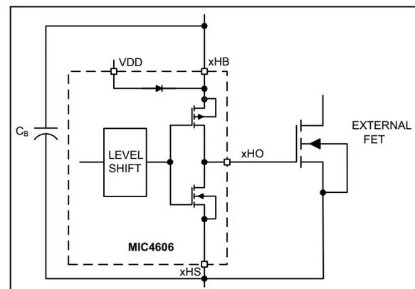
**FIGURE 6-2:** High-Side Driver and Bootstrap Circuit Block Diagram.
