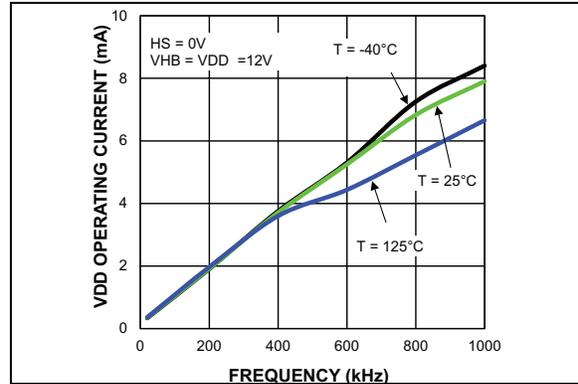
**FIGURE 3-16:**  $V_{DD}$  Operating Current vs. Frequency.
