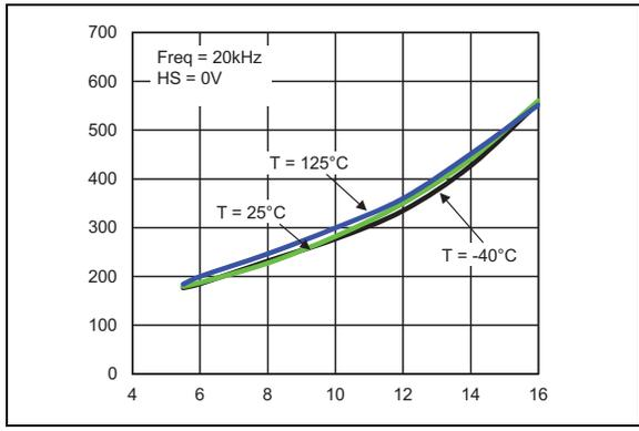
**FIGURE 3-3:**  $V_{DD}$  Operating Current vs. Input Voltage.
