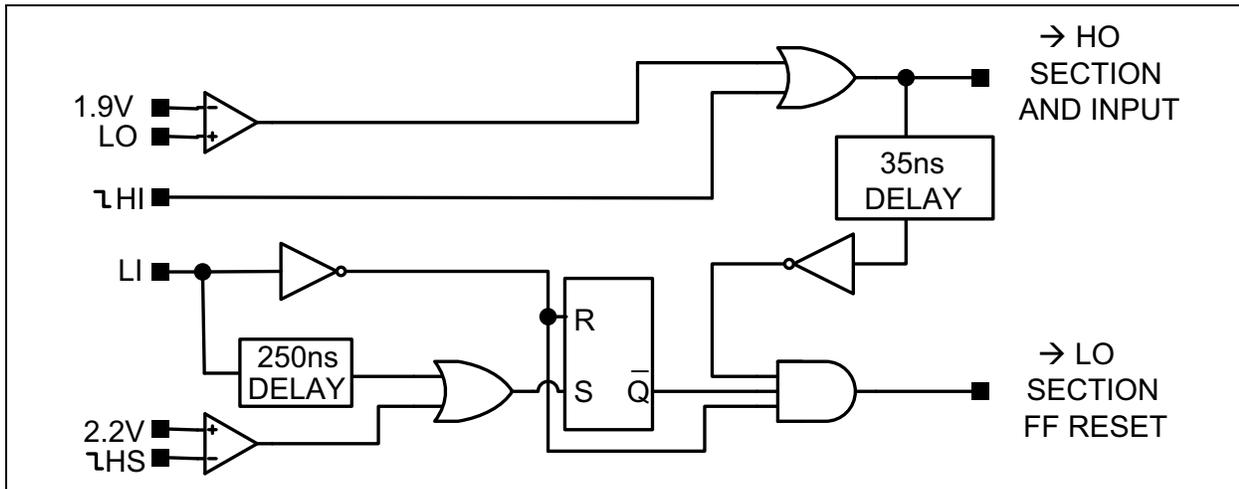
FIGURE 5-2: Input Logic Block in Figure 5-1.
