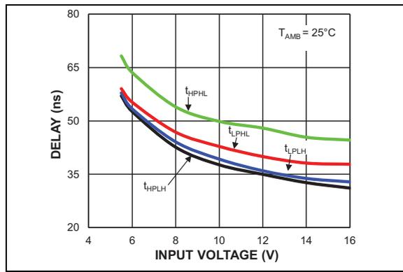
**FIGURE 3-5:** Propagation Delay vs. Input Voltage.
