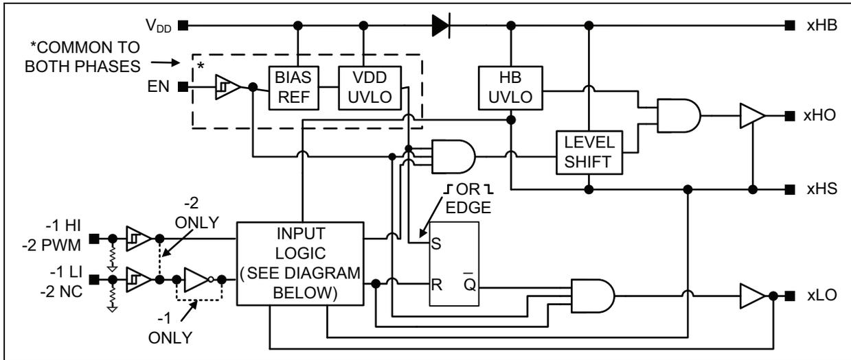
FIGURE 5-1: MIC4606 xPhase Top Level Block Diagram.
