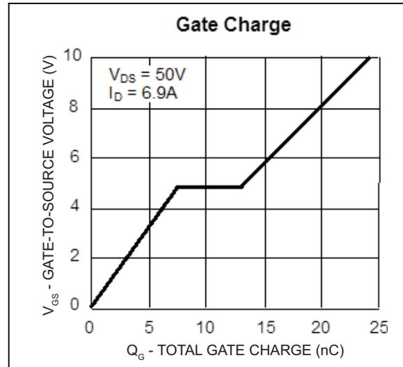
**FIGURE 7-8:** Typical Gate Charge vs.  $V_{GS}$ .
