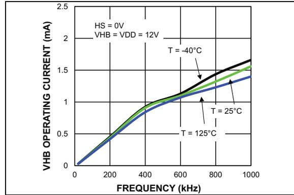
**FIGURE 3-17:**  $V_{HB}$  Operating Current vs. Frequency.
