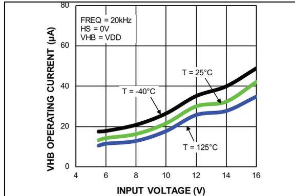
**FIGURE 3-4:**  $V_{HB}$  Operating Current vs. Input Voltage.
