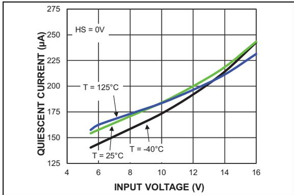
**FIGURE 3-1:**  $V_{DD}$  Quiescent Current vs. Input Voltage.
