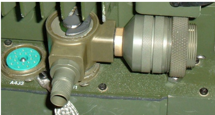
MPAUP/1-2A-2B0175 – The receptacle is oriented to the left as depicted above with the plug facing forward.
