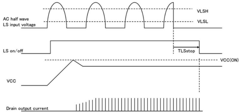
(B) Slow start and stop of LS start/stop mode (SO is connected to VDD)
