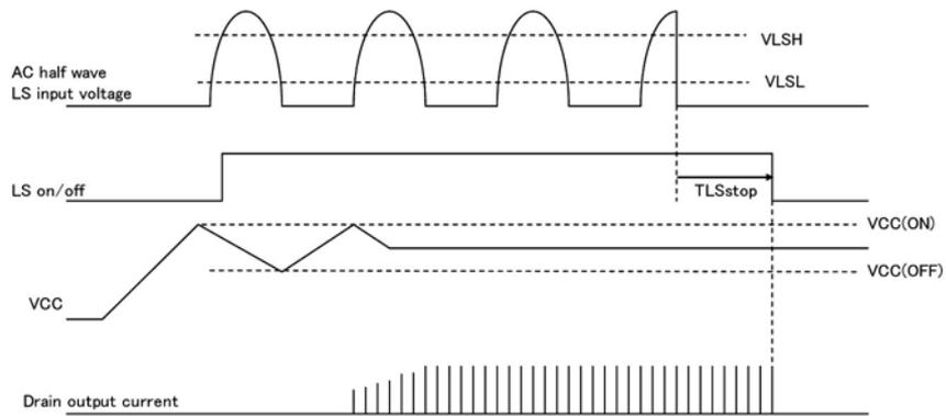
(C) Usual start and stop of LS detect SO signal mode (SO is connected to external parts)
