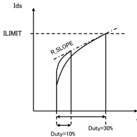
$$R_{\text{slope}} ; \{(\text{ILIMIT at Duty}=30\%) - (\text{ILIMIT at Duty}=10\%)\} / \{(\text{Ton at Duty}=30\%) - (\text{Ton at Duty}=10\%)\}$$
