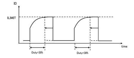
\* Load L, R during the ILIMIT measurement are: L=100uH, Rd=130 $\Omega$
