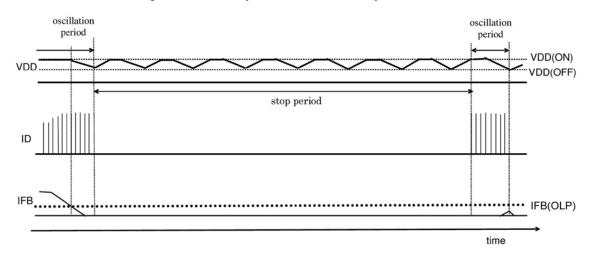
\*5 : Terminal waveforms when MAXDC is detected which makes timer intermittent operation becomes invalid Though FB current is below IFB(OLP) which indicates the detection of overload state, if the ON duty of the drain current is operating at MAXDC, drain oscillation will occur in every rise and fall cycle of the VDD terminal.
