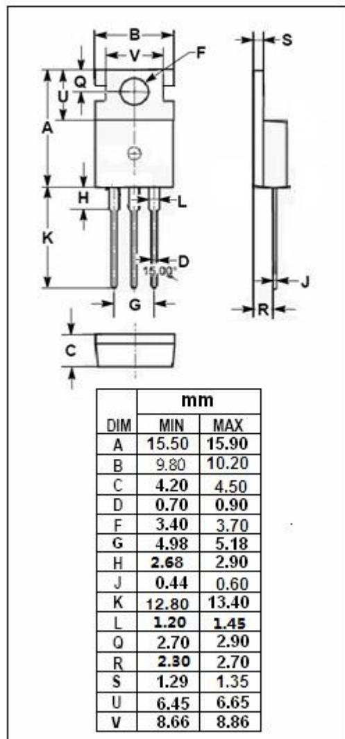
**isc Silicon NPN Power Transistor**
