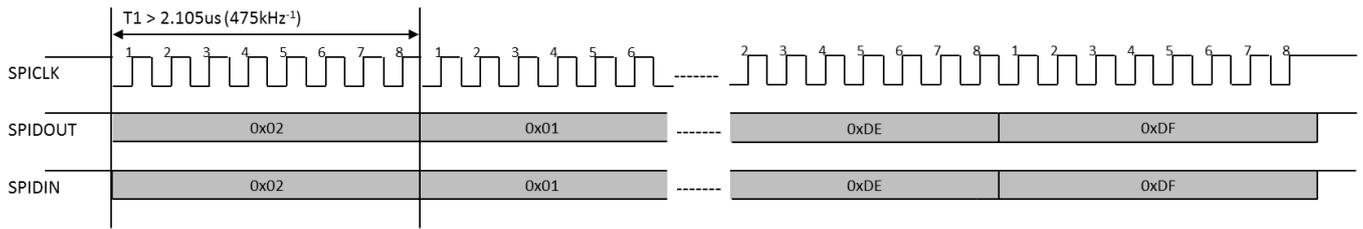
Time interval between byte transfer (t>0)
