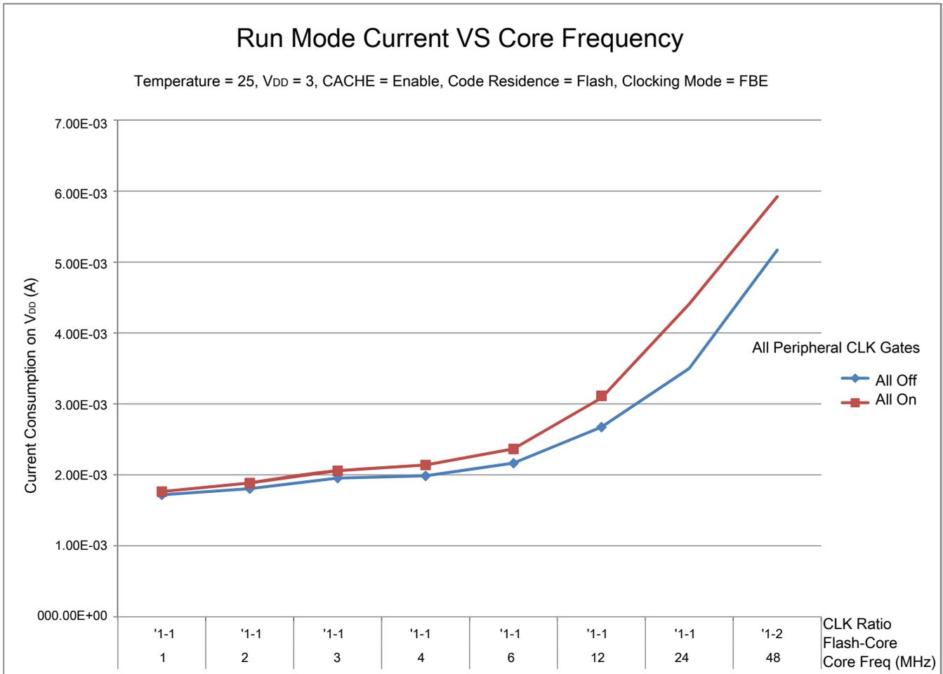
**Figure 1. Run mode supply current vs. core frequency**
