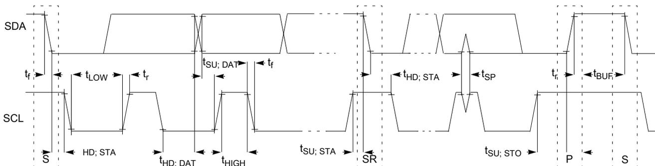
**Figure 16. Timing definition for fast and standard mode devices on the I<sup>2</sup>C bus**
