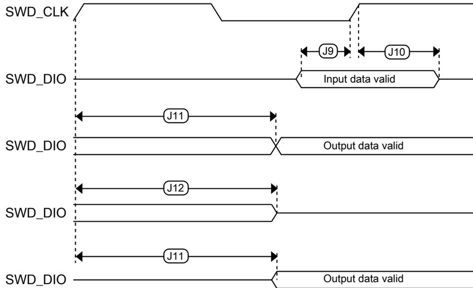
Figure 4. Serial wire data timing
