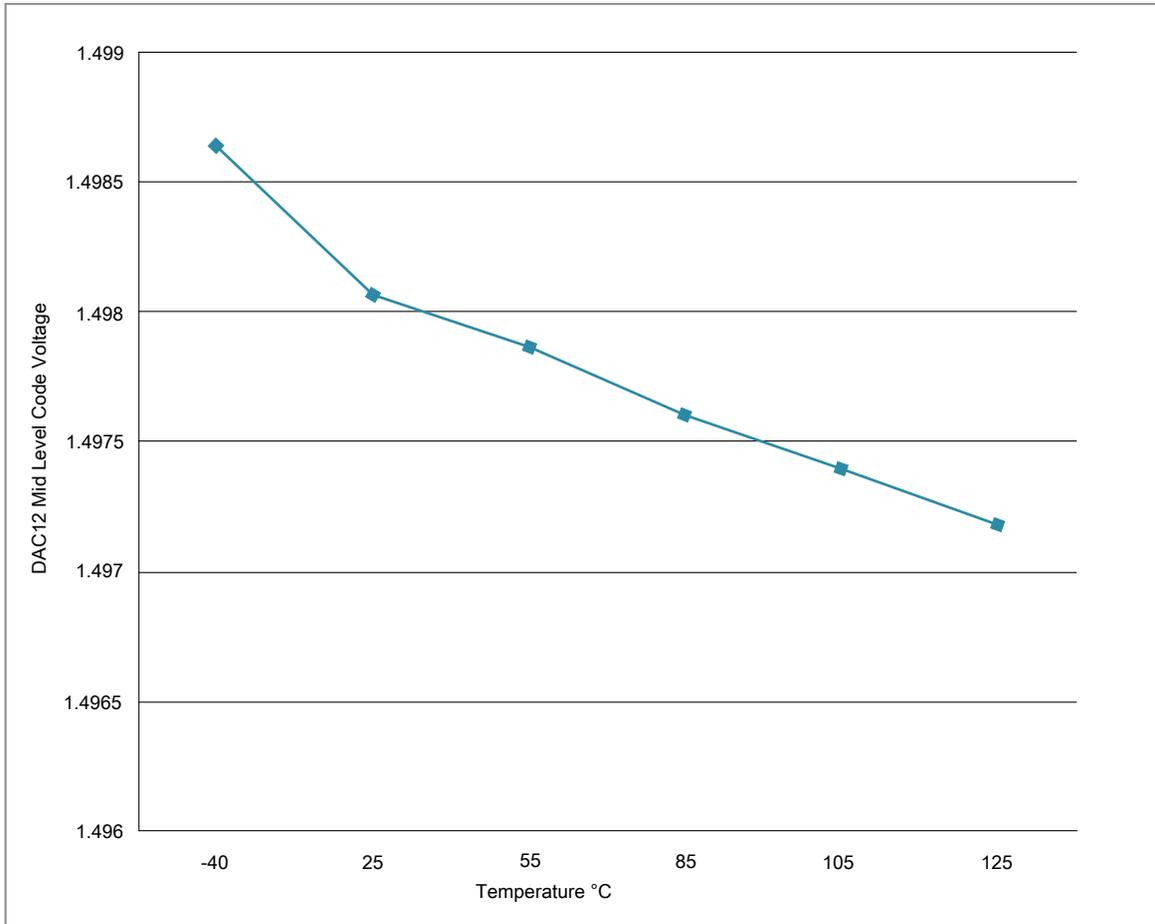
Figure 11. Offset at half scale vs. temperature
