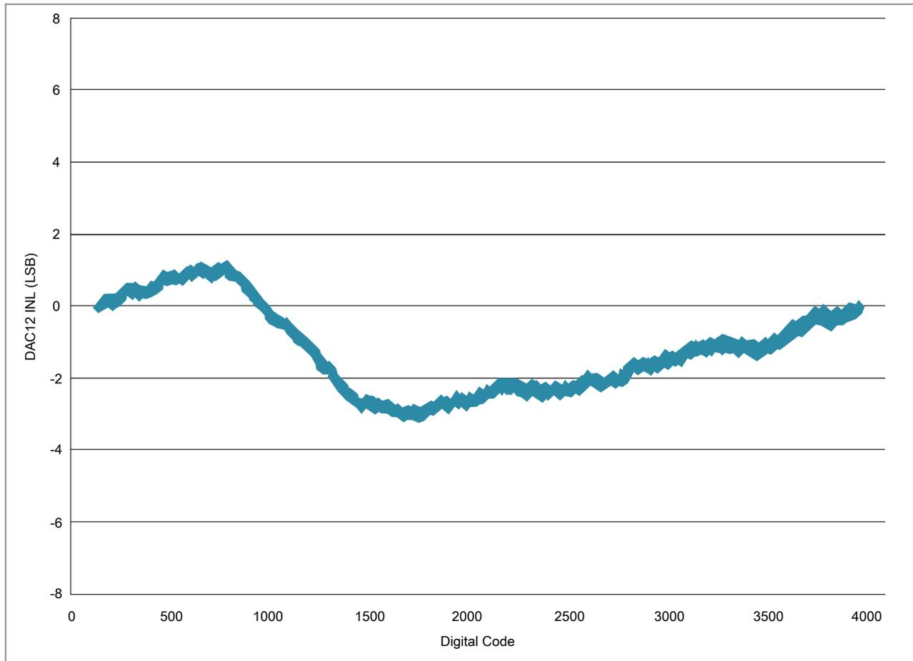
Figure 10. Typical INL error vs. digital code
