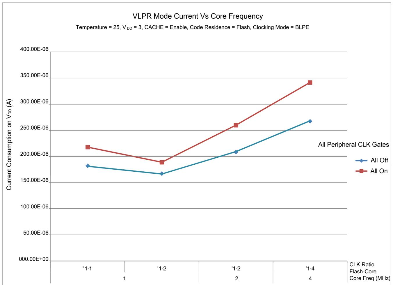
Figure 2. VLPR mode current vs. core frequency
