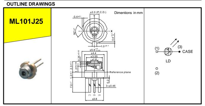
There is no model with a monitor photo diode in ML1XX25 series.
