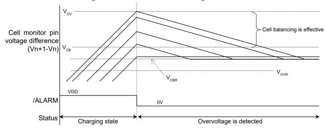
Cell balancing is executed at cells whose voltage is between over voltage detection threshold  $V_{\text{OV}}$  and cell balancing detection threshold  $V_{\text{CB}}$ .
