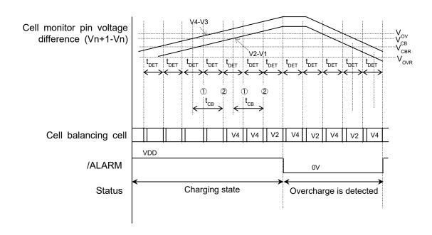
Cell balancing operation is shown below.
