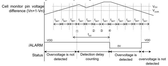
• In case if the overvoltage detection delay counting is initialized
