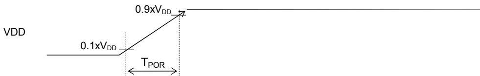
Power-on reset activation power rise time ( T_{POR} )
