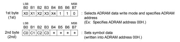
To specify symbol data continuously to the next address, specify only symbol data as follows. The address of ADRAM is automatically incremented. Specification of addresses is therefore unnecessary.
