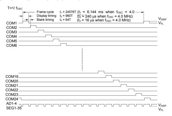
• Digit Output Timing (for 24-digit display, at a duty of 960/1024)
