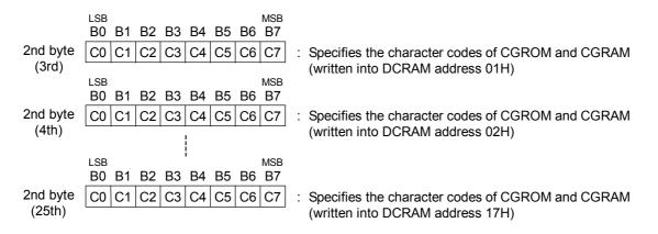
The character code setting of CGROM and CGRAM up to 24 digits is completed. To set a character code from DCRAM address 00H continuously. Specify a dummy character code between DCRAM addresses 18H and 1FH. (To increment the DCRAM address automatically and set it to 00H)
