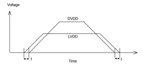
If LVDD is in the range of 0 V to LVDDmin, make sure that  $LVDD \ge DVDD$  and  $t \ge 0[ns]$  are satisfied. When performing power-on reset with a capacitor connected to the RESET pin, be careful about the relationship between the capacitance value and the rise time of the power supply.
