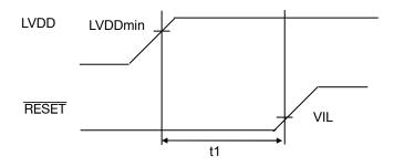
Drive the  $\overline{\text{RESET}}$  pin Low and hold it Low under the condition "t1  $\ge$  0[ns]" until LVDD reaches LVDDmin.
