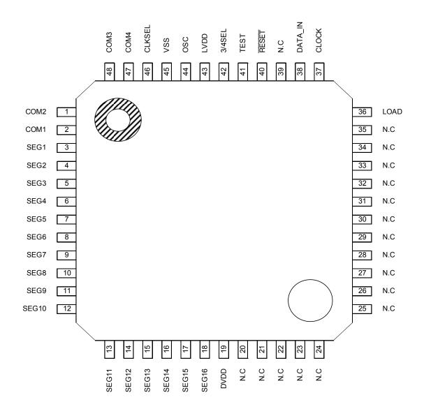
48-Pin Plastic TQFP
