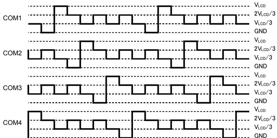
● Common segment output waveform
