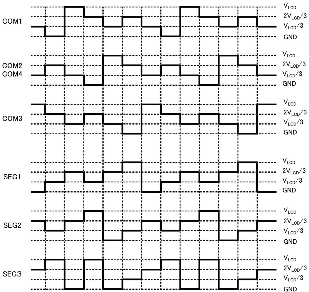
● Common and segment output waveforms
