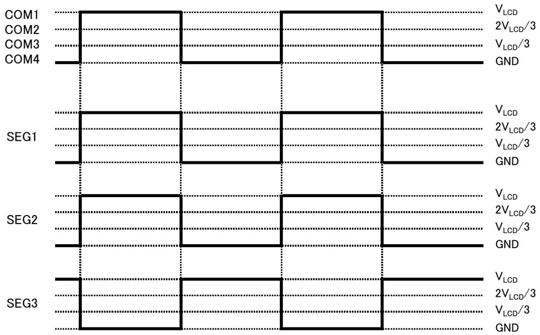
● Common and segment output waveforms
