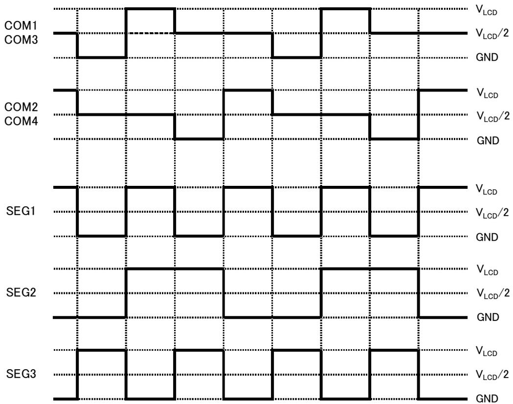
● Common and segment output waveforms
