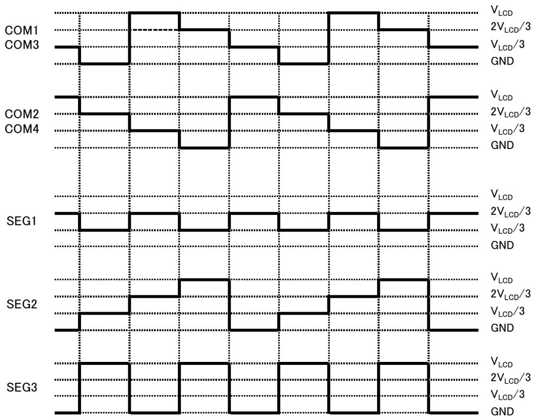
● Common and segment output waveforms
