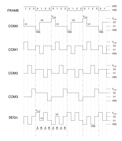
note: In this mode, the signal of COM4 is same as the 'FRAME' signal shown below.
