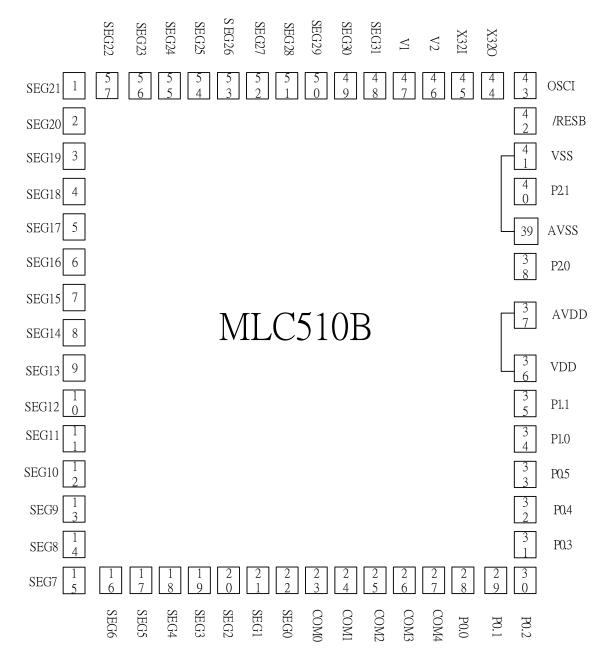
Note: AVDD must connect to VDD, and AVSS must connect to VSS
