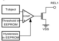
The comparator is a digital comparator, with a resolution of 12 bits. By default the input polarity is inverting. Threshold and hyteresis values are version dependent, as indicated below. These settings can be changed by factory programming on request.
