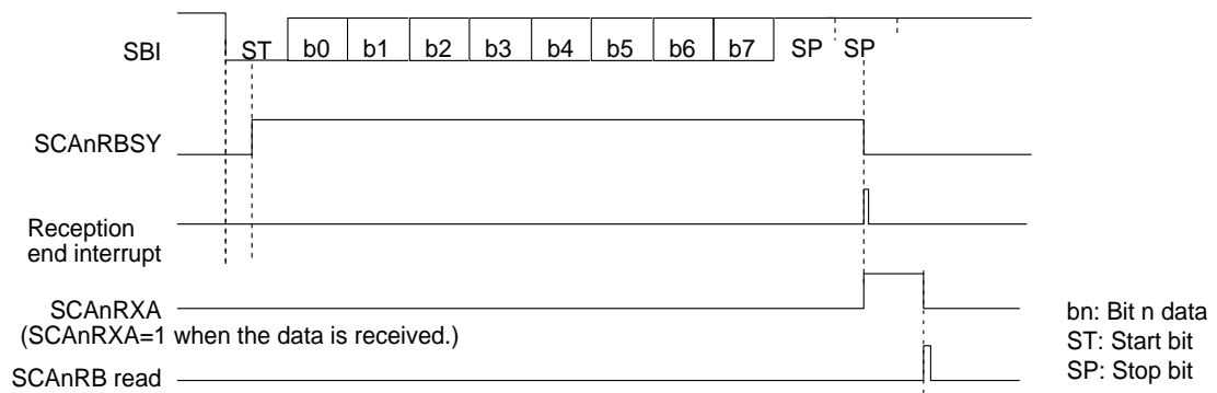
Figure 6-3-7 Asynchronous Reception Timing
