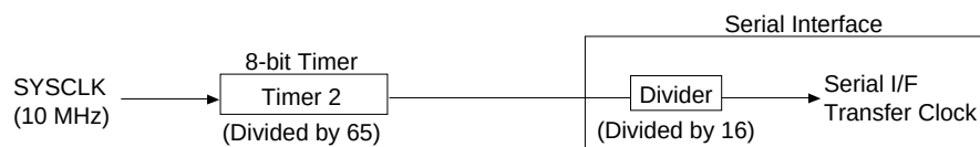
Figure 5-2-1 Asynchronous Transmission Configuration
