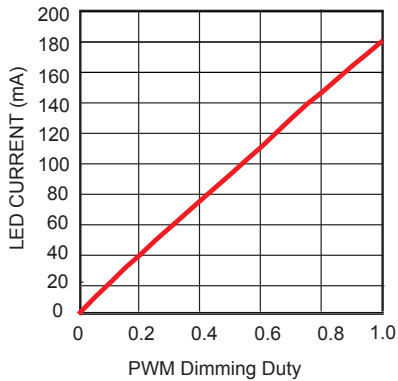
LED Current vs. PWM Dimming Duty
