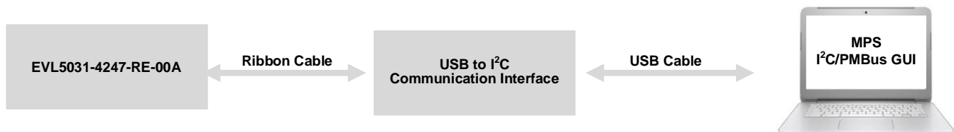
Figure 1: EVKT-MP5031 Evaluation Kit Set-Up
