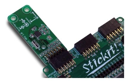
Inserting Into a Wing Socket
